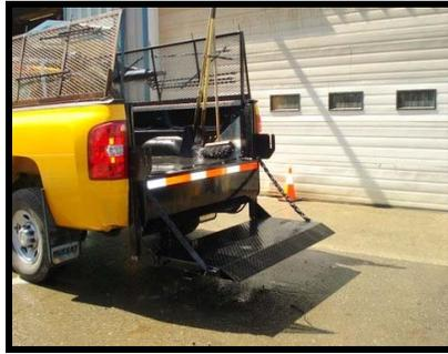
Emcon continues to upgrade the fleet with this new Power Tailgate on a 3/4 ton pickup. This will allow the crews to safely lift heavy loads.
